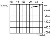
FIG.2 REVERSE CURRENT VS. REVERSE VOLTAGE
